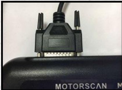
1.Connect the main test cable cable
